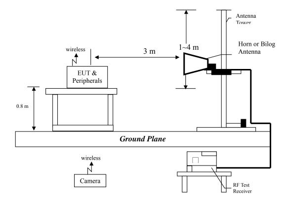
Radiated emission measurements were performed from 30MHz to 25GHz. Spectrum Analyzer Resolution Bandwidth is 100kHz or greater for frequencies 30MHz to 1GHz, 1MHz – for frequencies above 1GHz.
