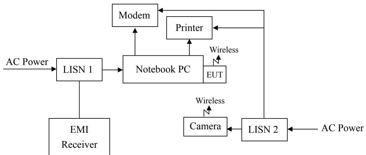
**The test procedure was according to ANSI C63.4/2003.**
