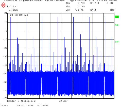
Number of pulses observed in 720ms=7 @ channel 0, 2408.625 MHz
