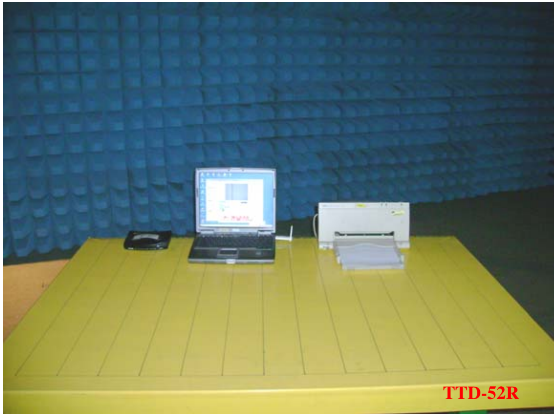
Photo 1: Radiated Emission Test set-up photo
