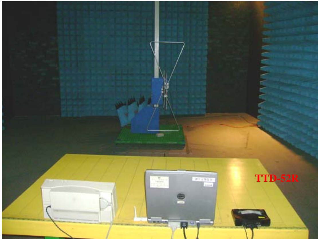
Photo 2: Radiated Emission Test set-up photo
