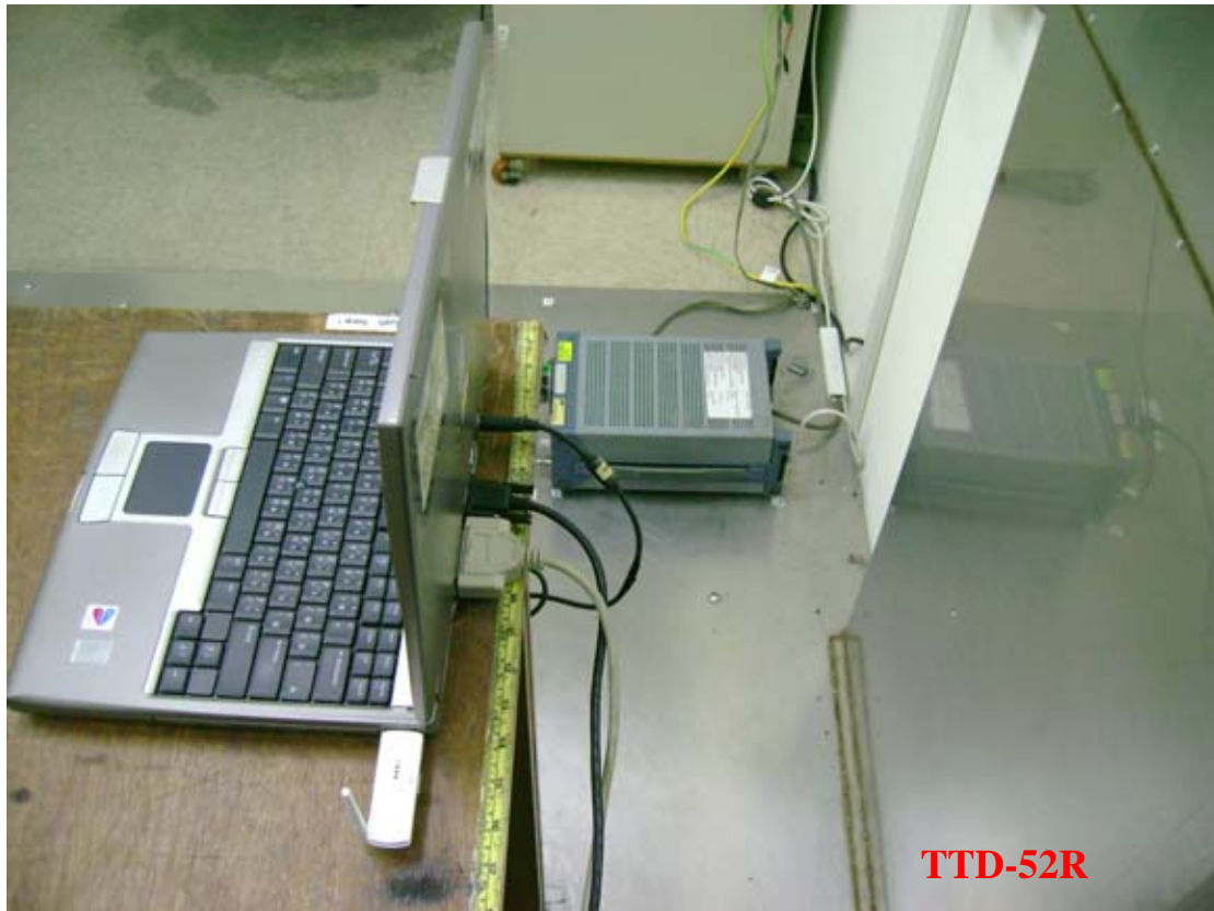
Photo 2: Conducted Emission Test Set-up photo
