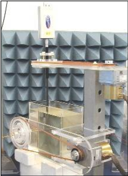
Figure 1. Spherical isotropy jig showing probe, dipole and box filled with simulated brain liquid (see Ref [2], Section A.5.2.1)
