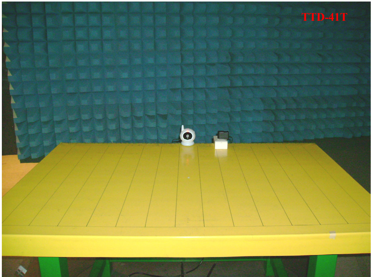
Photo 1: Radiated Emission Test set-up photo
