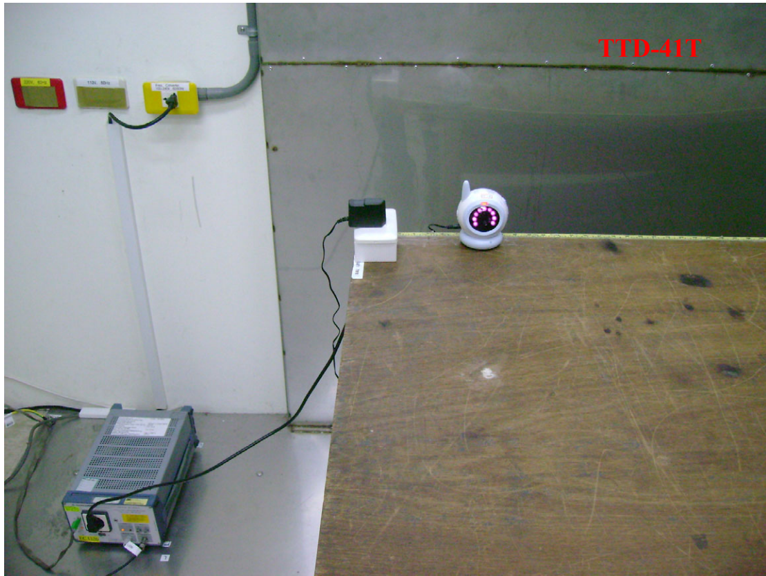
Photo 1: Conducted Emission Test Set-up photo
