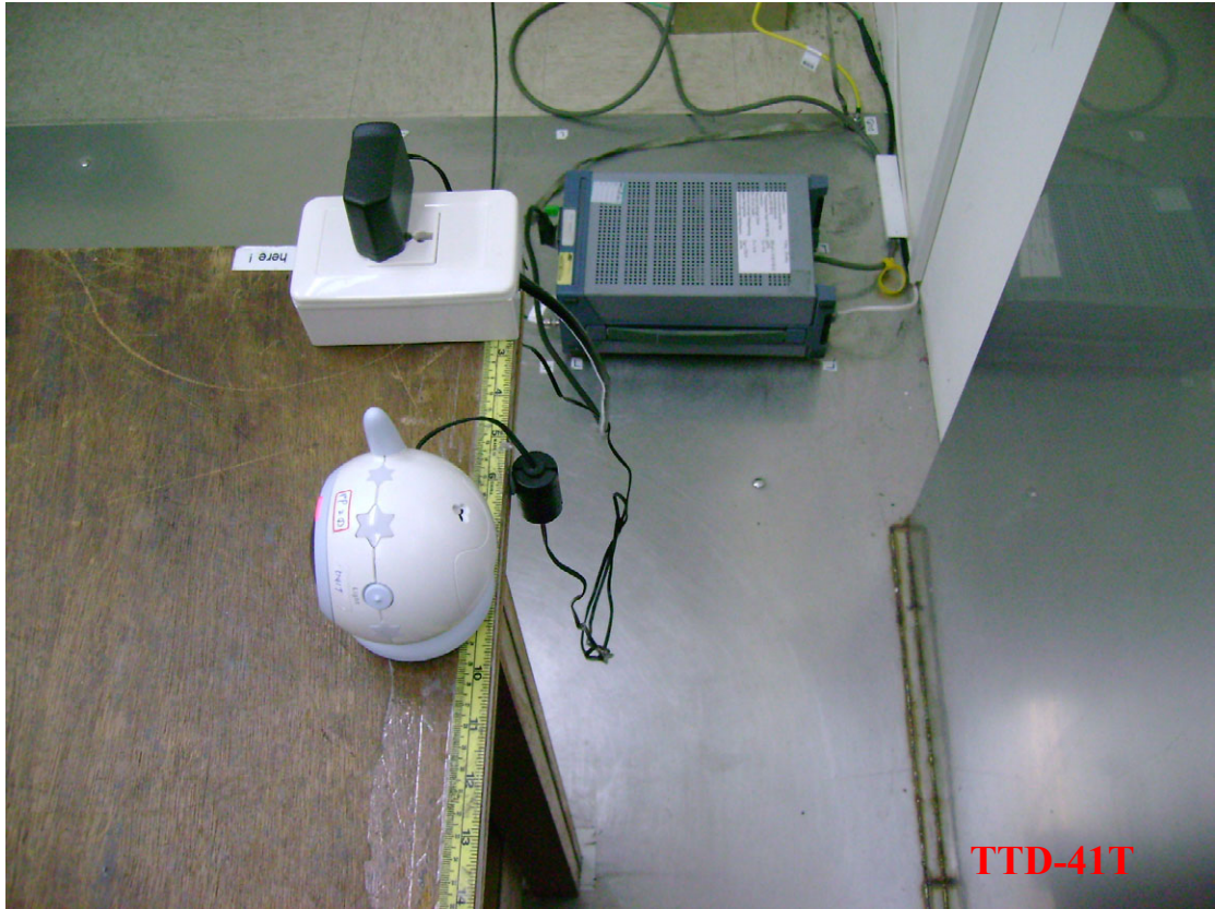
Photo 2: Conducted Emission Test Set-up photo
