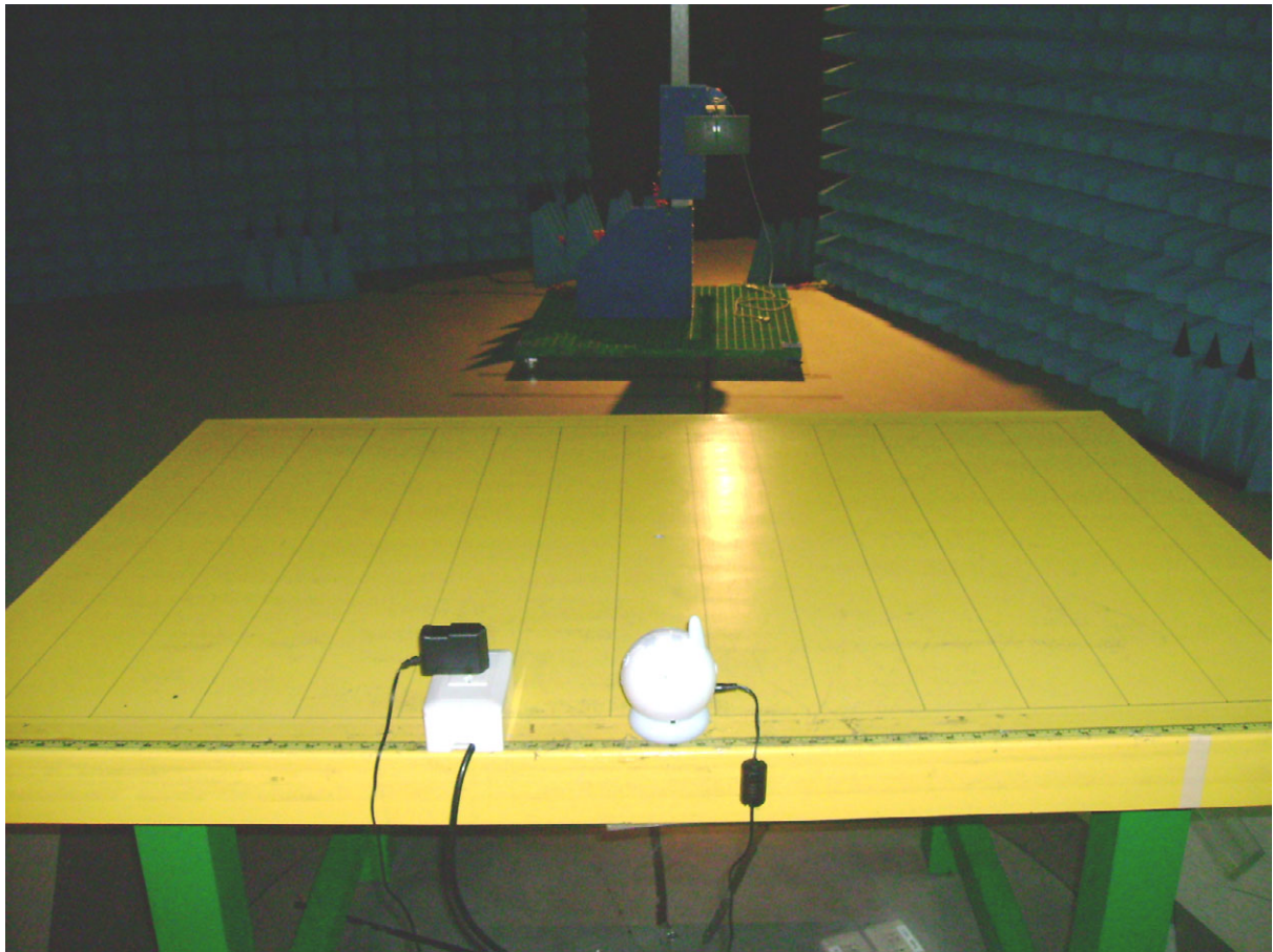
Photo 4: Radiated Emission Test set-up photo
