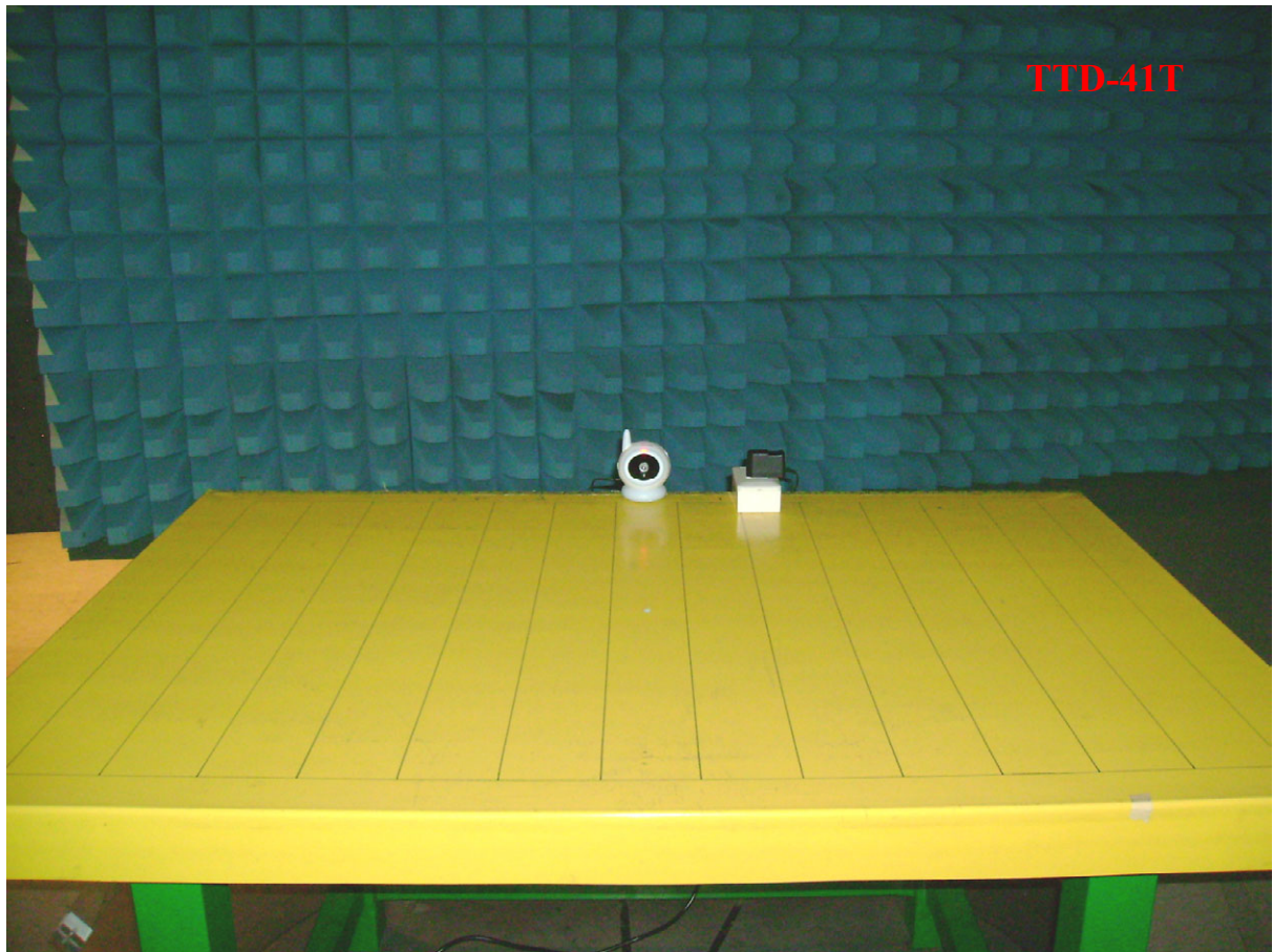
Photo 3: Radiated Emission Test set-up photo
