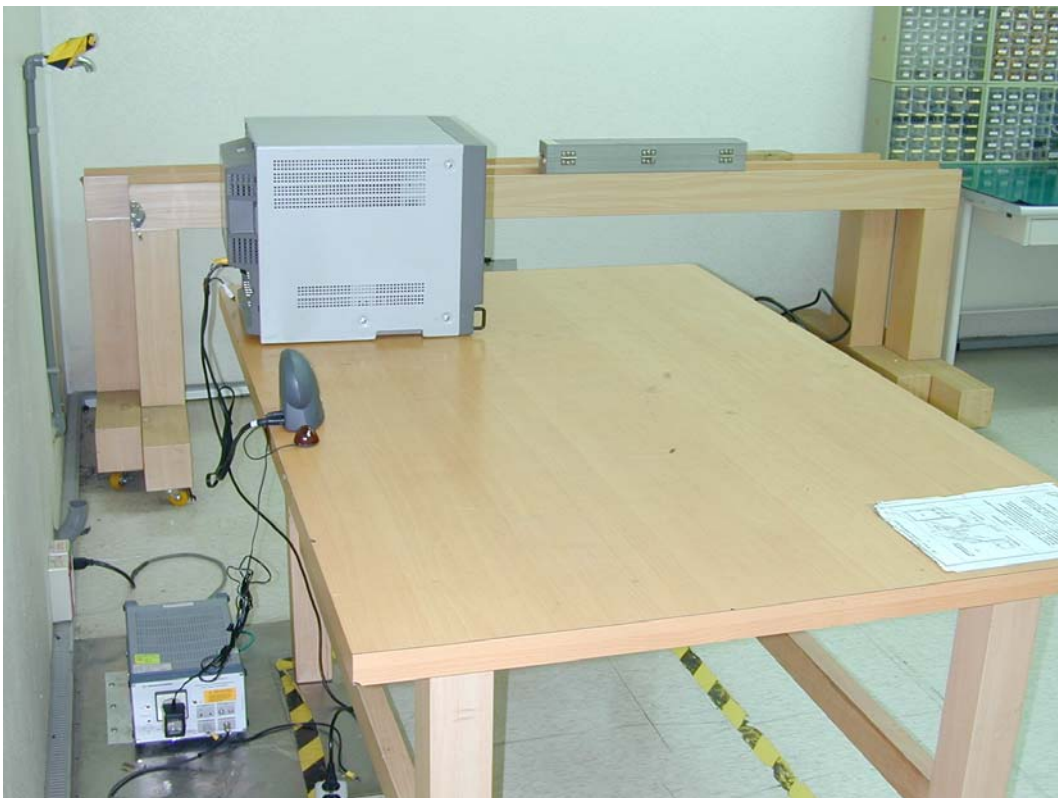
Back View of Conducted Test (Adapter: AC adapter)
