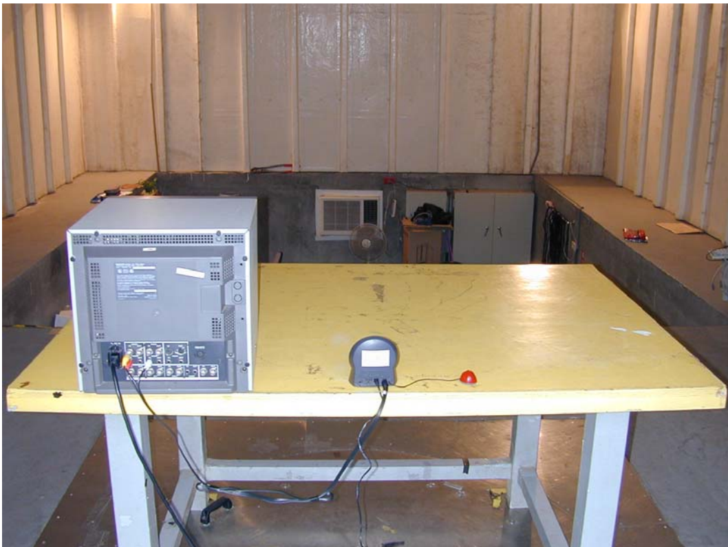
Back View of Radiated Test (Adapter: AC adapter)
