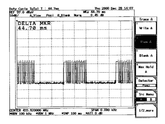
PEAK= 75.22dBuV/m; Duty Cycle= 20 LOG (12.4/44.7); Average= Peak +Duty Cycle= 64.08
