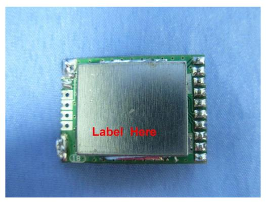
The Label of FCC ID number will be placed on the RF module as shown in the photograph below:
