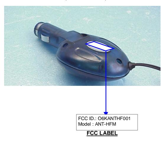
[Mark]: Due to size of the equipment, the label contains only the FCC ID. and the compliance statement is provided in the User's Manual.
