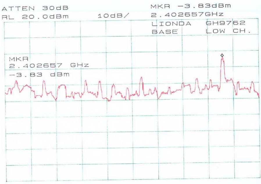
CENTER 2.402300GHz \*ABW 3.0KHz \*VBW 3.0KHz SPAN 1.000MHz \*SWP 1.0Ksec
