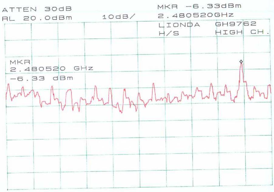
CENTER 2.480130GHz \*ABW 3.0KHz \*VBW 3.0KHz \*SWP 1.0Ksec
