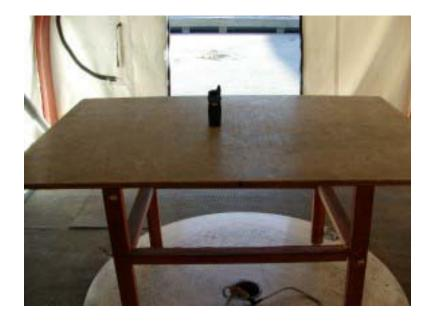
**Handset Radiated Emission - Rear View**
