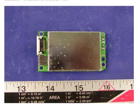
**Handset - Transceiver Cover Removed Component View**
