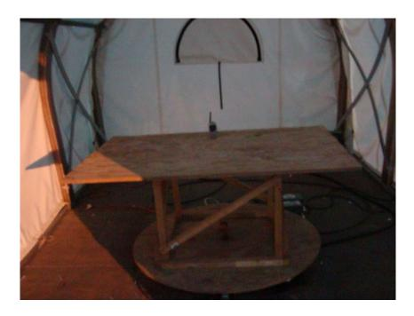
**Radiated Emission Setup - Rear View**
