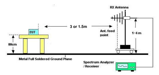
Above 10 GHz shall be extrapolated to the specified distance using an extrapolation factor of 20 dB/decade from 3m to 1.5m.
