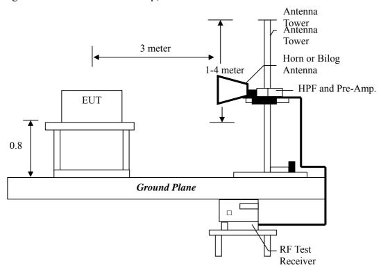
Radiated emissions were invested cover the frequency range from 30MHz to 1000MHz using a receiver RBW of 120kHz record QP reading, and the frequency over 1GHz using a spectrum analyzer RBW of 1MHz and 10Hz VBW record Average reading. (15.209 paragraphs), the Peak reading (1MHz RBW/VBW) recorded also on the report.
