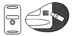
2. Press the connect button of the USB Dongle.
