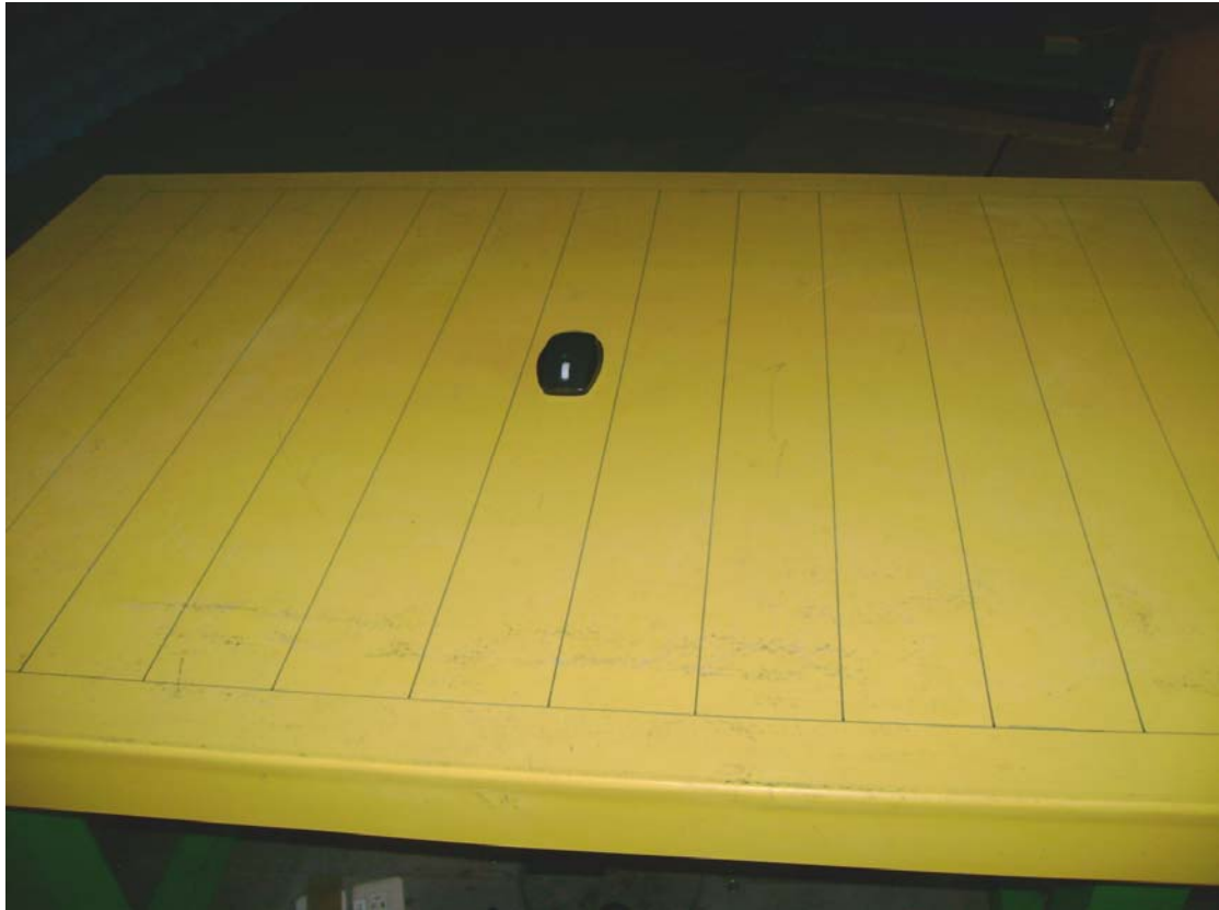
Photo 2: Radiated Emission Test set-up photo
