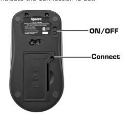
**Notes**: You only need to connect the mouse and keyboard to the receiver for the first time. The mouse and keyboard will store the connection into memory for later use.
