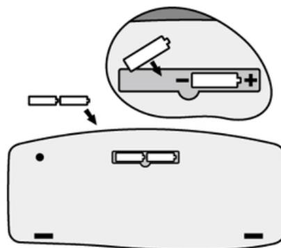
**NOTE:** After replacing batteries, please refer to **Section 3 - Establishing a Wireless Connection** to re-establish the wireless connection.
