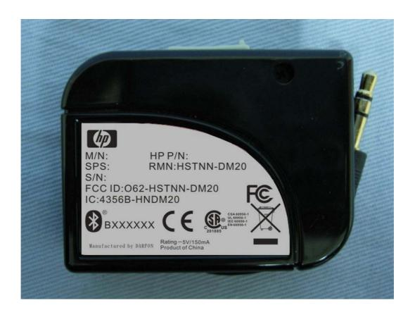
The IC ID Label will be placed on the equipment as shown in the photograph below.
