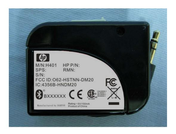
The IC ID Label will be placed on the equipment as shown in the photograph below.
