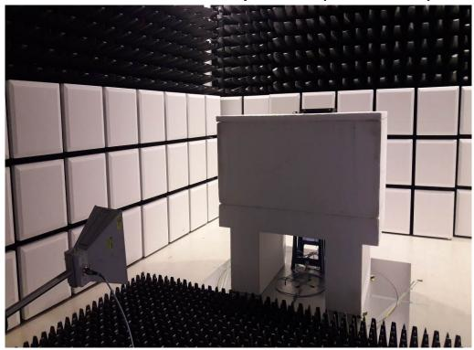
Radiated Emission Set up Photos (Front View)
