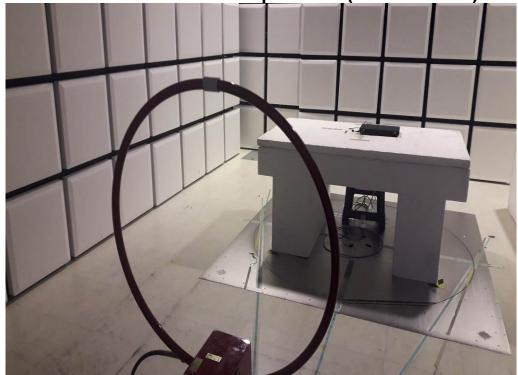
Radiated Emission Set up Photos (Below 1GHz)
