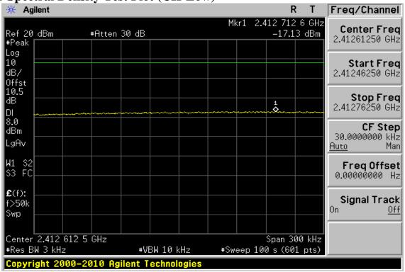
**Power Spectral Density Test Plot (CH-Mid)**
