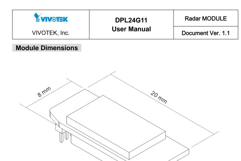
All dimensions are in millimeters. Tolerance: +/- 0.15mm
