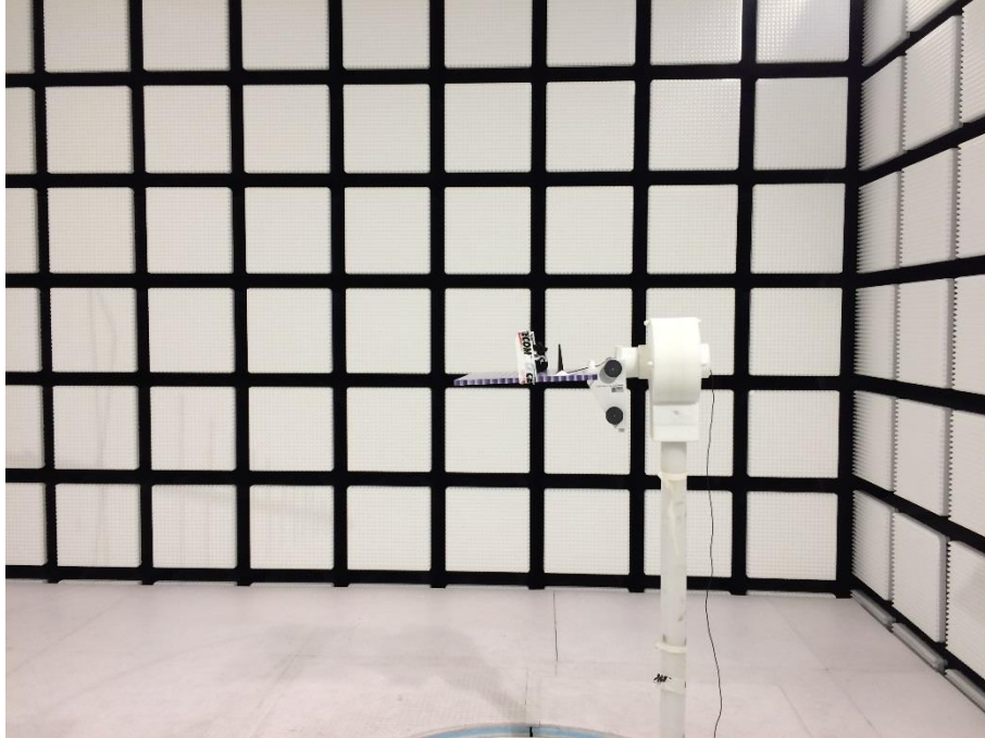
Photo 1 (RSE set-up / fully-anechoic chamber):
