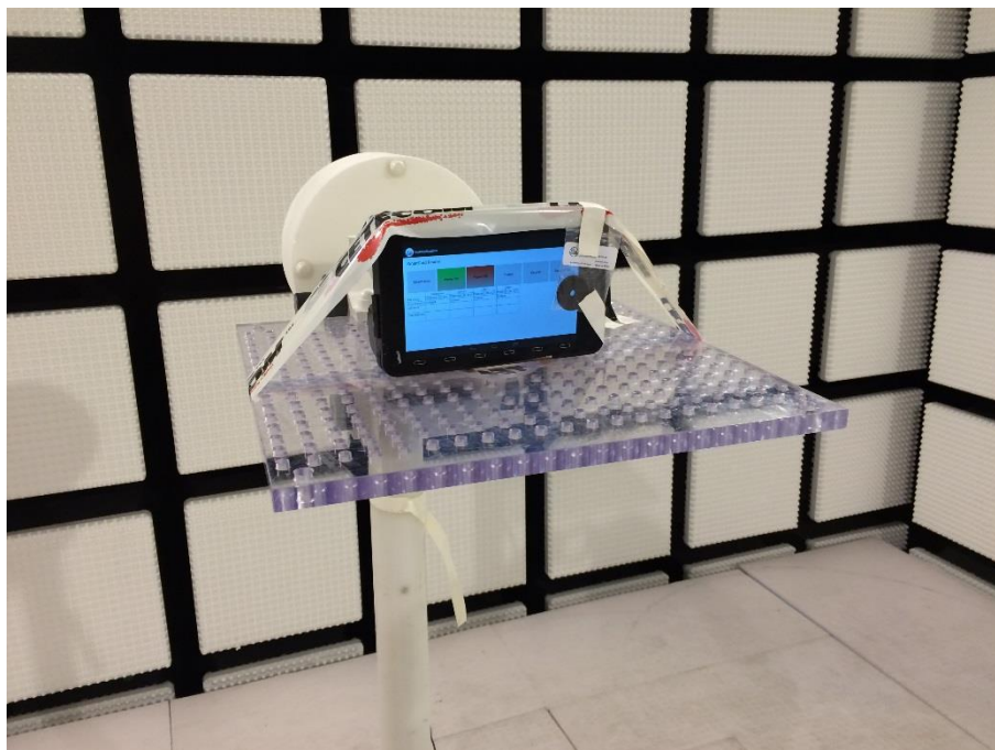
Photo 4 (RSE set-up / fully-anechoic chamber):
