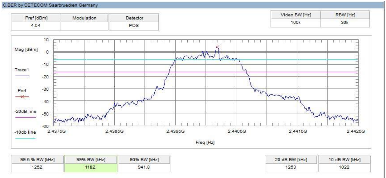
Plot 5: middle channel – 2441 MHz, Pi / DQPSK modulation
