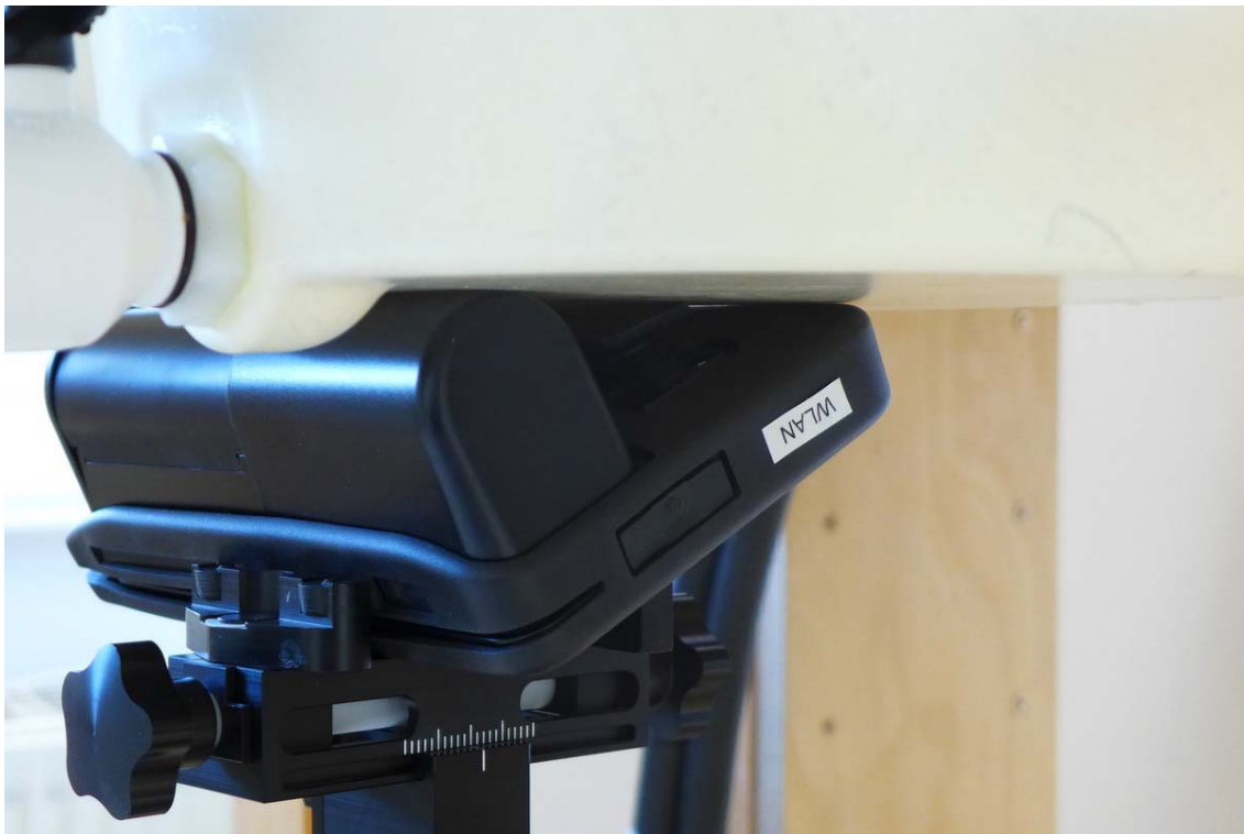
Fig. 25: Back side towards the phantom, 0 mm distance, WLAN antenna.
