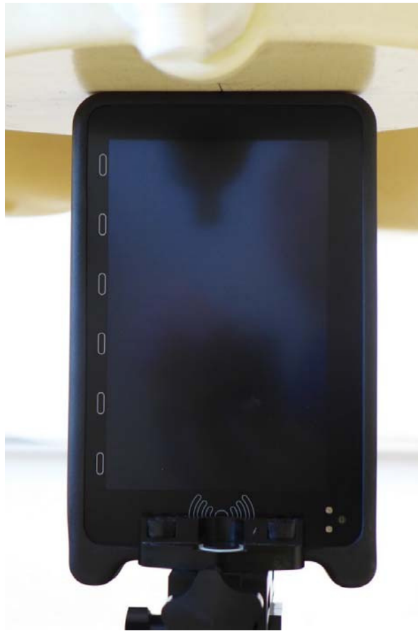
Fig. 24: Right side towards the phantom, 0 mm distance, WLAN antenna.
