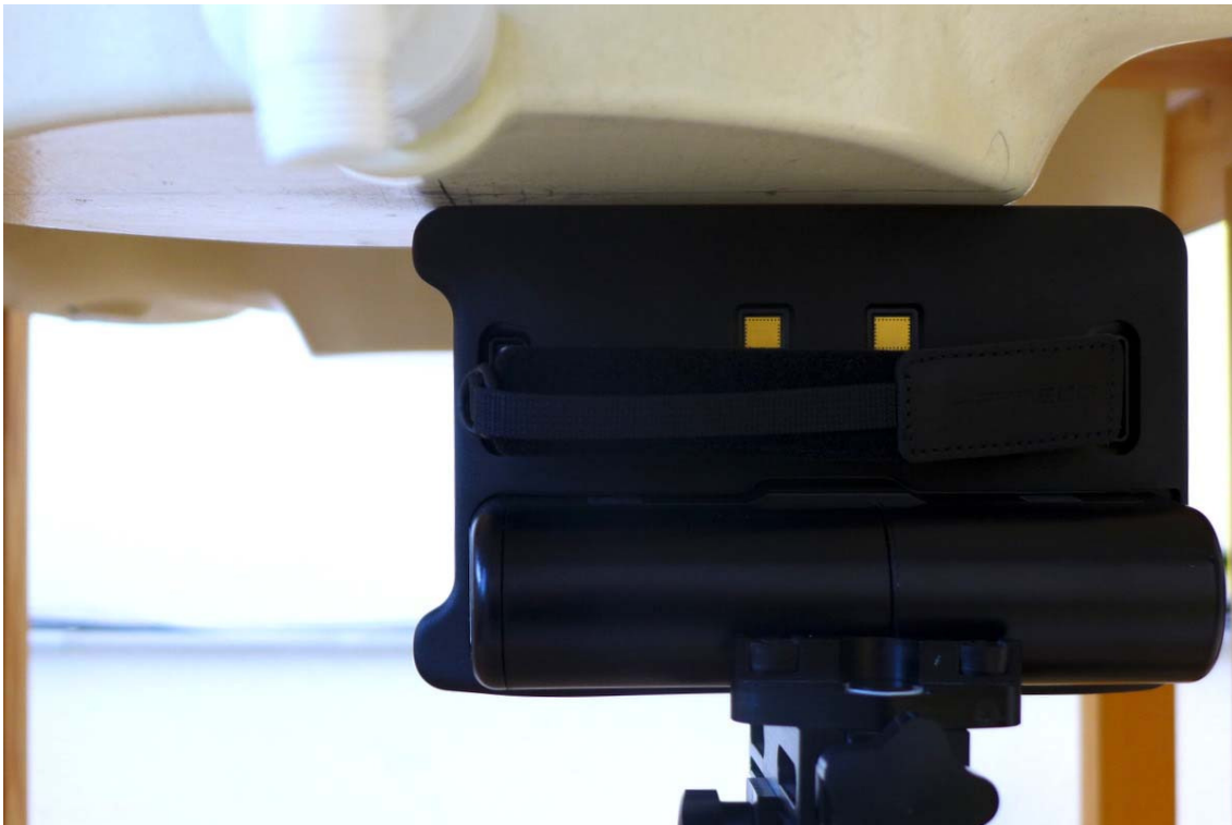
Fig. 21: Bottom side towards the phantom, 0 mm distance, WWAN antenna.
