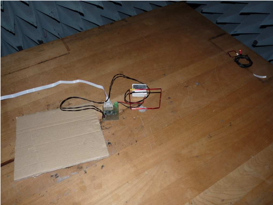
Photo 4: Setup_04, radiated measurements (below 30 MHz) Antenna ANTd01 (04184970)
