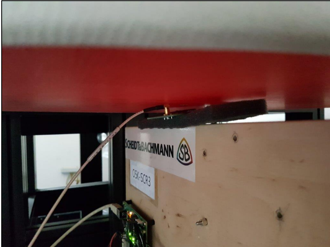
Photo 9: Test position - Antenna 2 - Back side with 0mm distance
