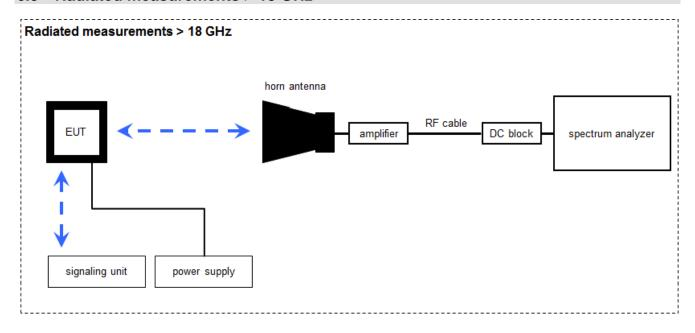
Measurement distance: horn antenna 50 cm
