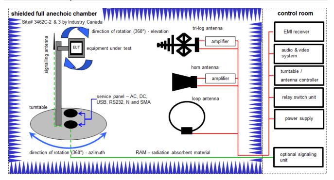
Measurement distance: tri-log antenna and horn antenna 3 meter; loop antenna 3 meter / 1 meter
