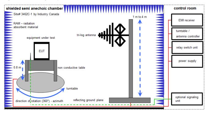
Measurement distance: tri-log antenna 10 meter
