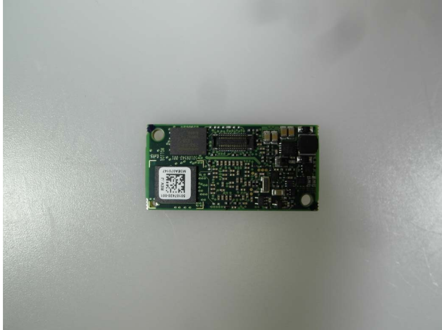
Photo 53: additional board optical sensor back side SV51
