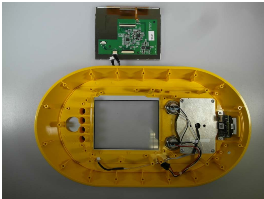
Photo 44: top cover back side and display back side SV51
