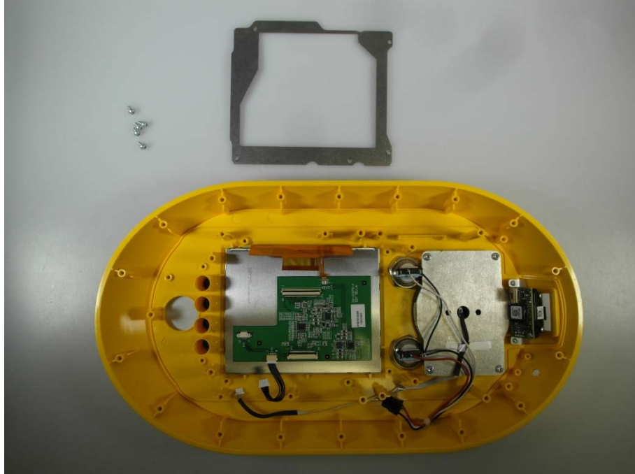
Photo 43: additional board with display electronic SV51
