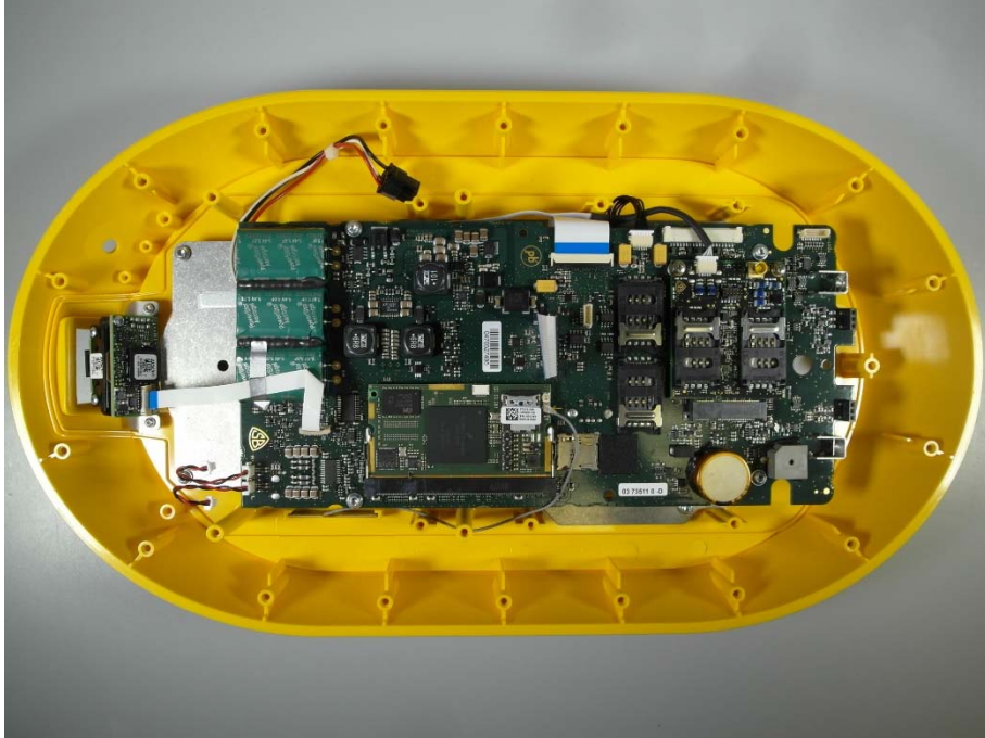
Photo 33: main board with additional Wi-Fi board SV51
