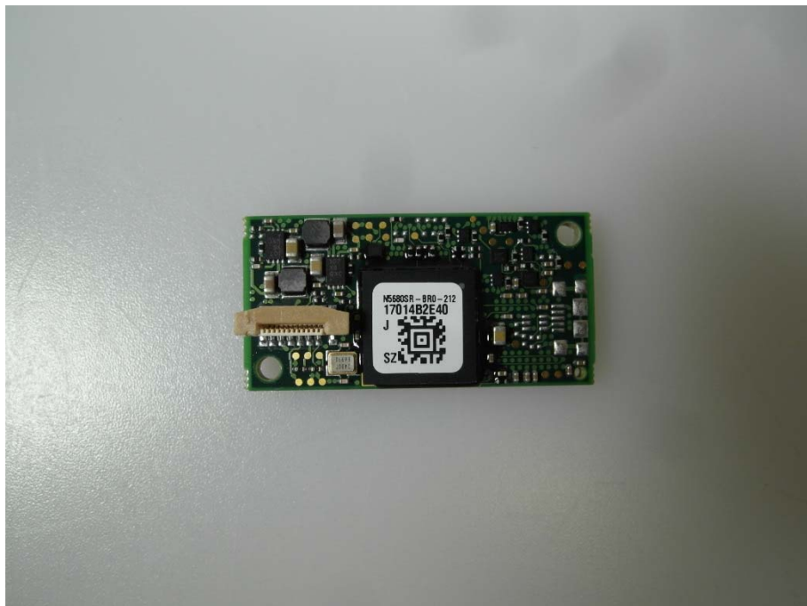
Photo 52: additional board optical sensor front side SV51
