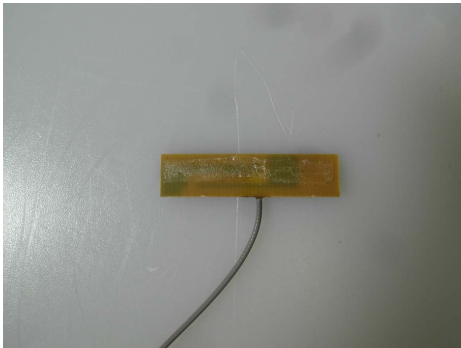
Photo 38: Wi-Fi antenna back side OV41/ SV51
