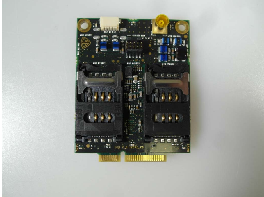
Photo 39: additional board with SIM card slots top side SV51
