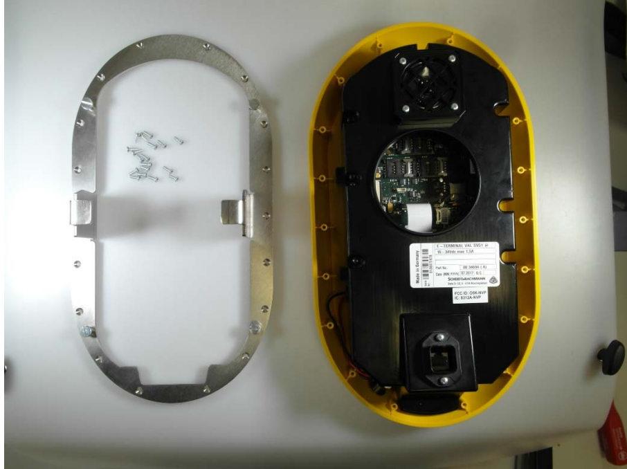
Photo 23: back side and mounting SV51
