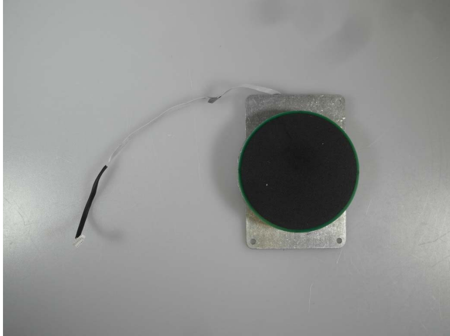
Photo 51: RFID antenna front side SV51
