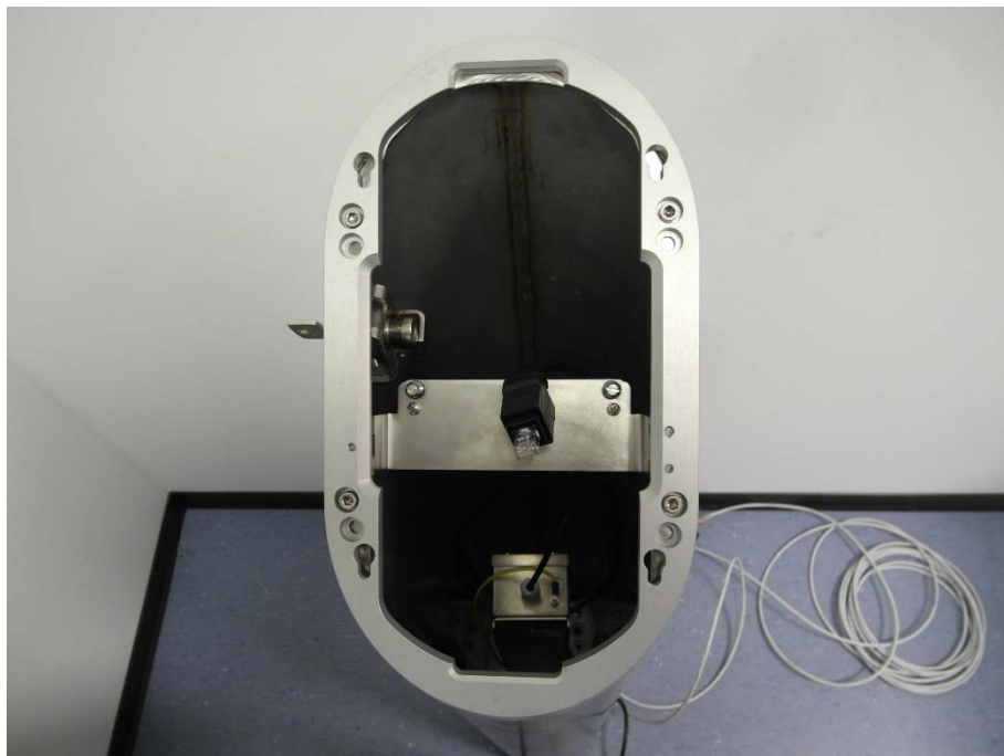
Photo 18: stand inside with LAN connector SV51
