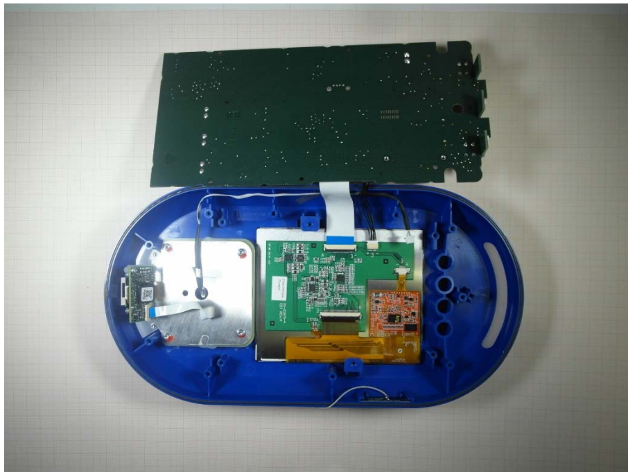
Photo 14: case with mainboard back side OV41
