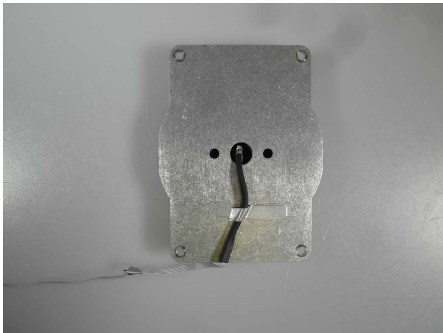
Photo 50: RFID antenna back side SV51
