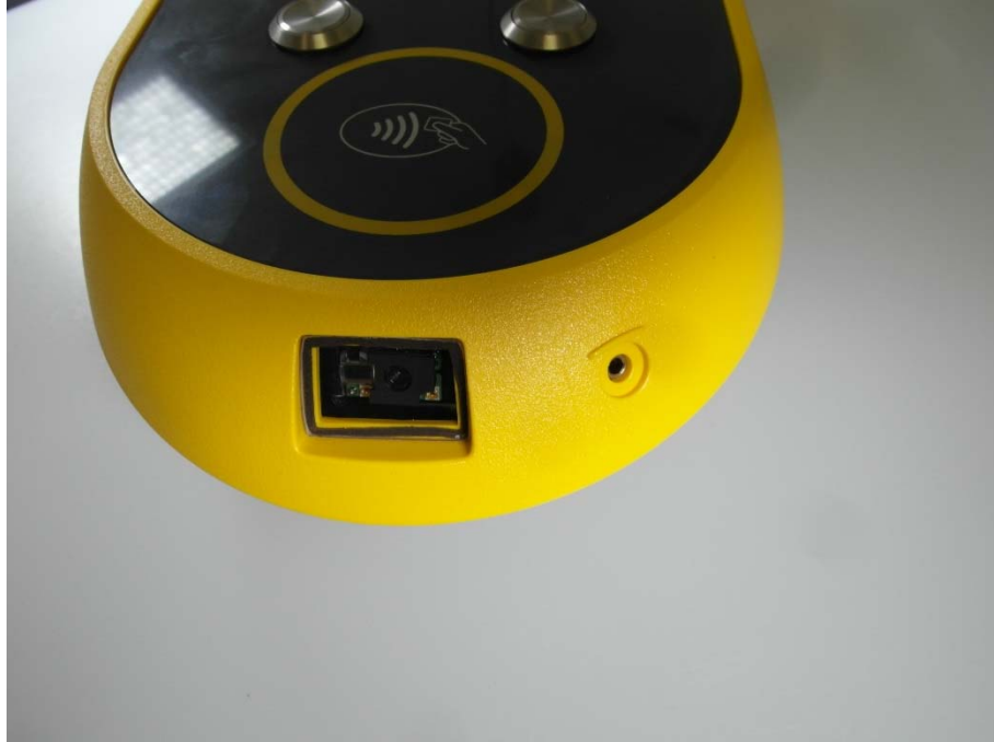
Photo 25: power connector and optical sensor outside SV51
