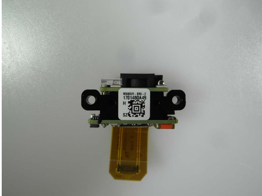
Photo 57: optical sensor top side SV51
