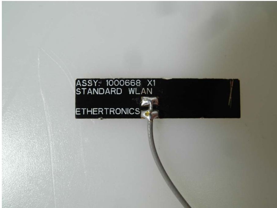
Photo 37: Wi-Fi antenna top side OV41 / SV51
