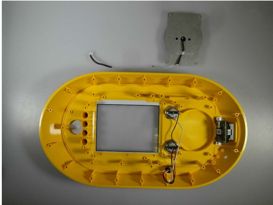
Photo 49: top cover and RFID antenna SV51
