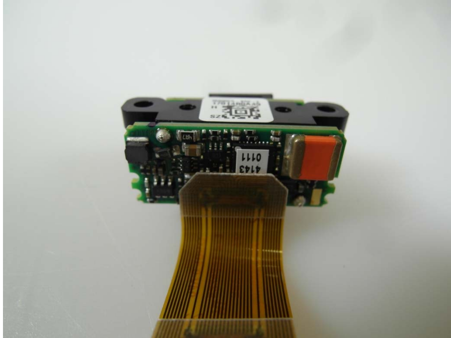
Photo 55: optical sensor back side SV51
