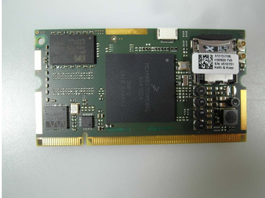
Photo 35: additional Wi-Fi board top side SV51
