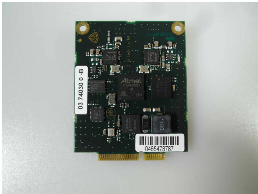
Photo 40: additional board with SIM card slots back side SV51
