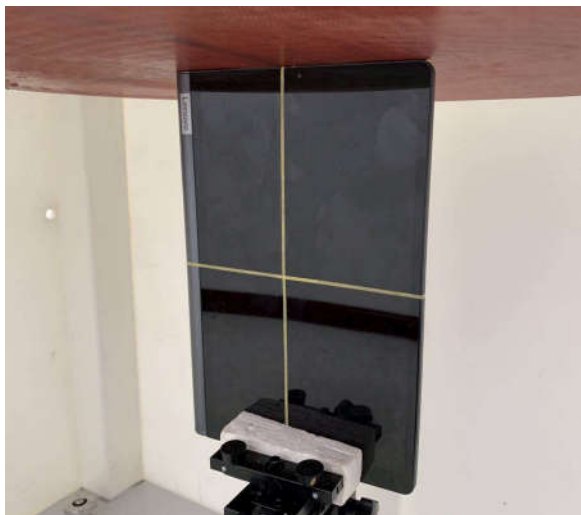
Edge4, Test Separation 0 mm
