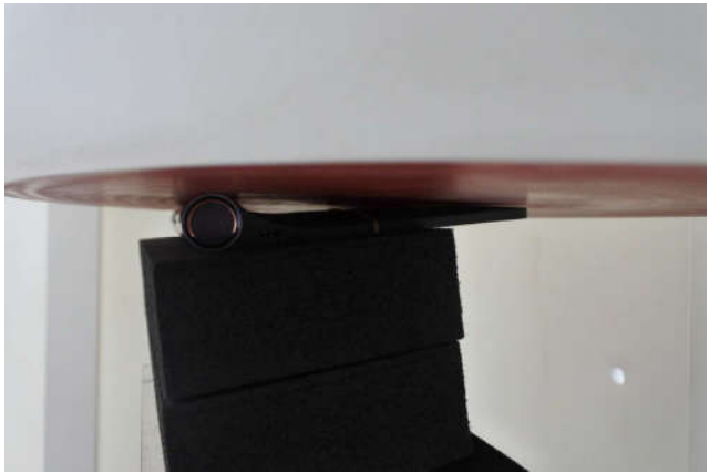
WLAN Bottom Face, Test Separation 0 mm
