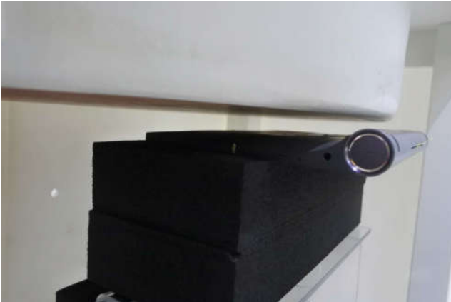
WWAN Bottom Face, Test Separation 15 mm
