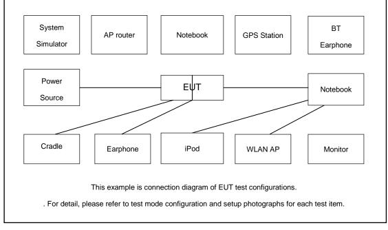
The EUT has been associated with peripherals pursuant to ANSI C63.4-2014 and configuration operated in a manner tended to maximize its emission characteristics in a typical application
