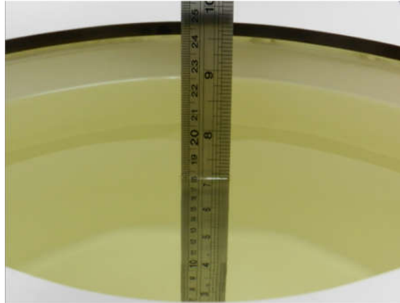
Fig 11.1 Photo of Liquid Height for Body SAR
