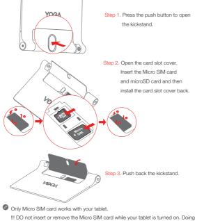
III DO not insert or remove the Micro SIM card while your tablet is turned on. Doing so can permanently damage your Micro SIM card or tablet.
