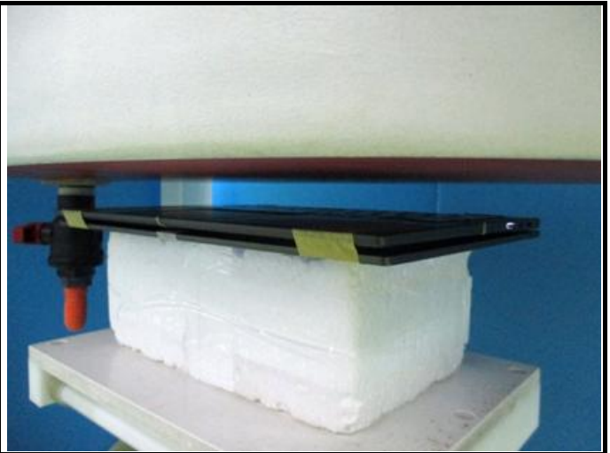
Body - Rear Face of EUT at 25 mm
