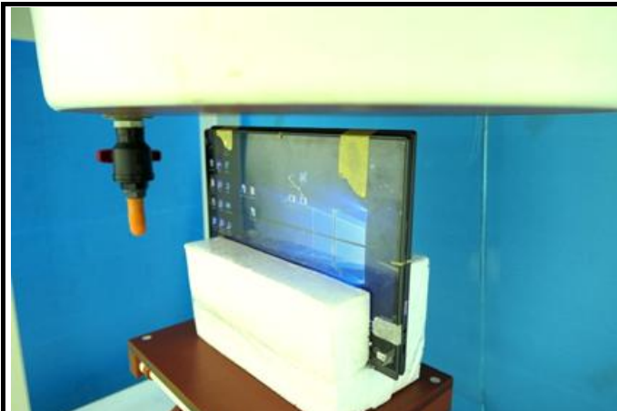
Body - Top Side of EUT at 13 mm
