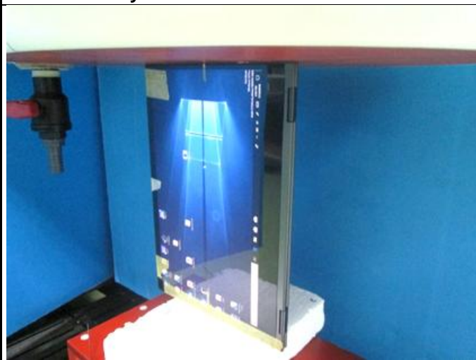
Body - Right Side of EUT at 0 mm
