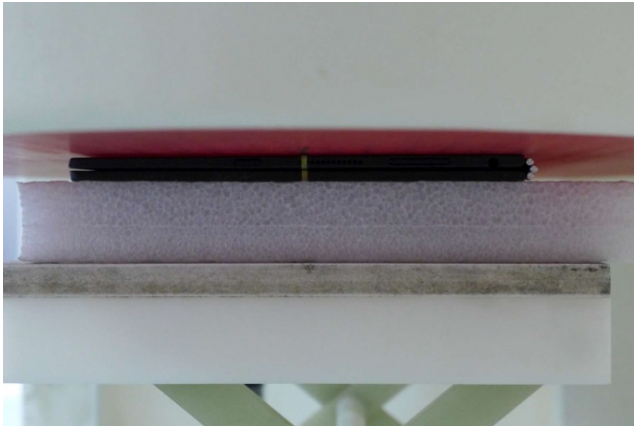
Bottom Face, Test Separation 0 mm
