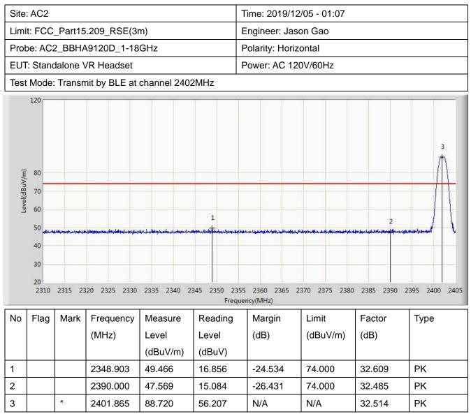
Note: Measure Level (dB $\mu$ V/m) = Reading Level (dB $\mu$ V) + Factor (dB)
