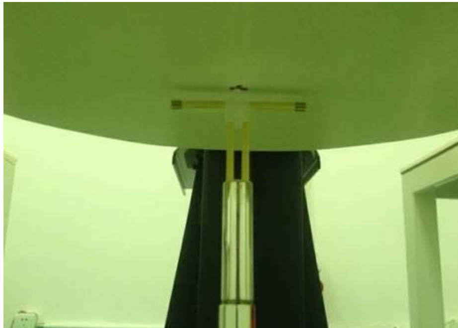
Picture 8.2 Photo of Dipole Setup
