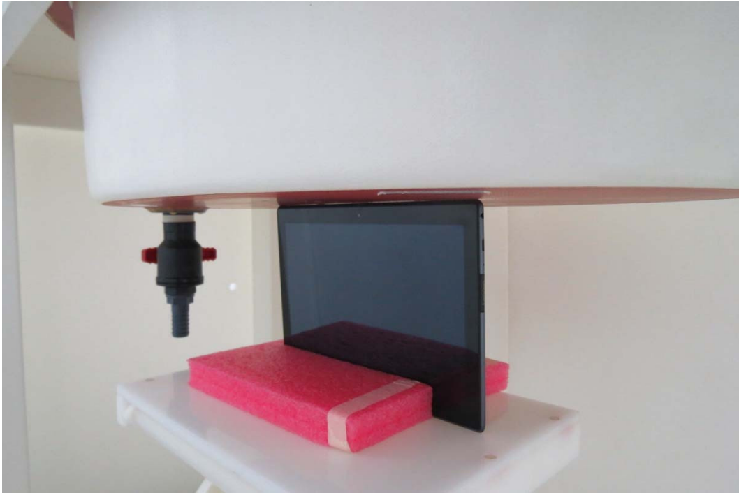
Picture 10: Top Edge, the distance from handset to the bottom of the Phantom is 0mm
