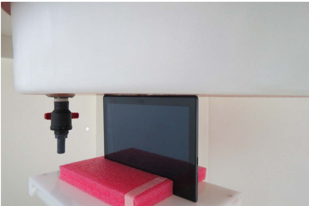
Picture 11: Bottom Edge, the distance from handset to the bottom of the Phantom is 14mm
