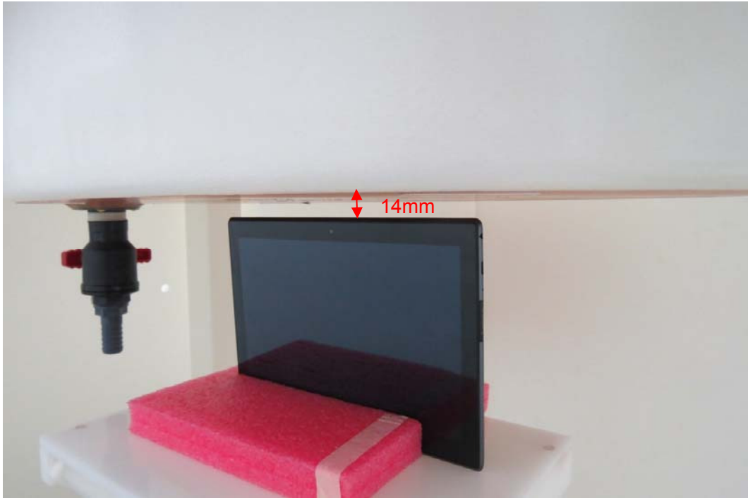
Picture 14: Top Edge, the distance from handset to the bottom of the Phantom is 14mm
