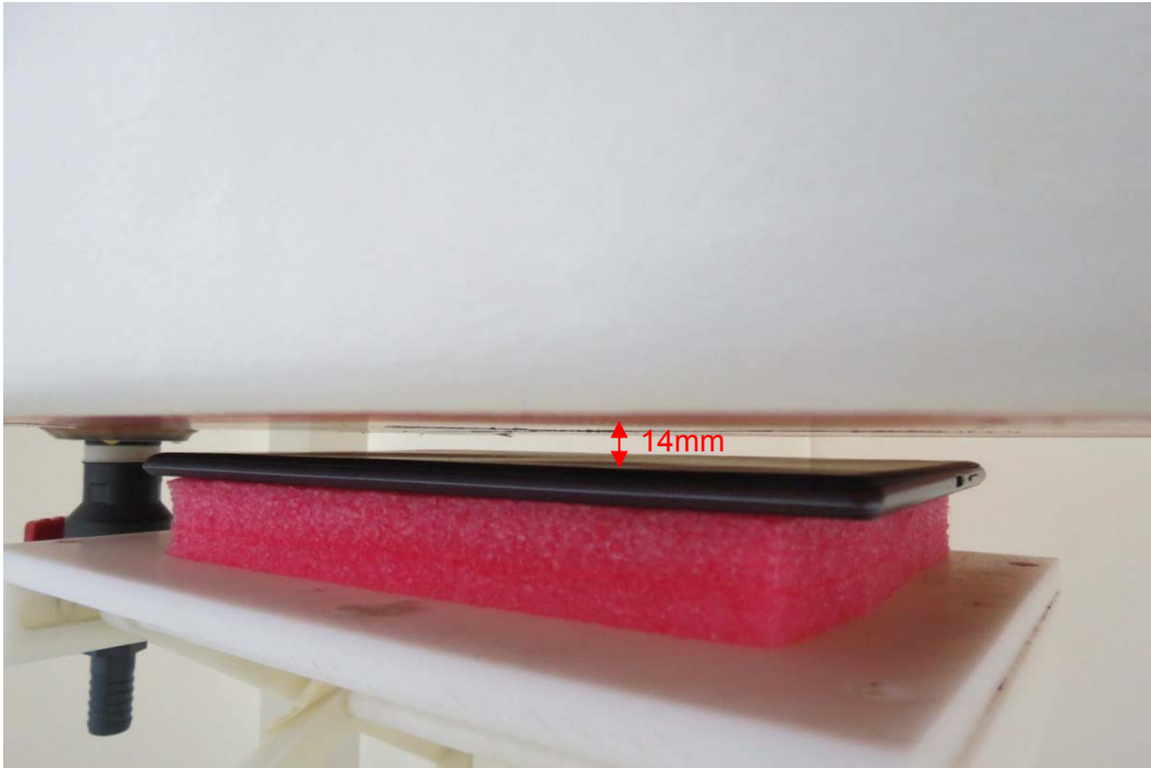
Picture 12: Back Side, the distance from handset to the bottom of the Phantom is 14mm
