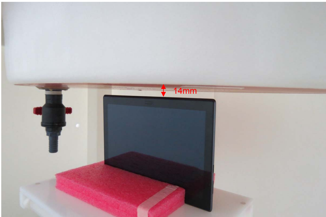
Picture 15: Bottom Edge, the distance from handset to the bottom of the Phantom is 14mm
