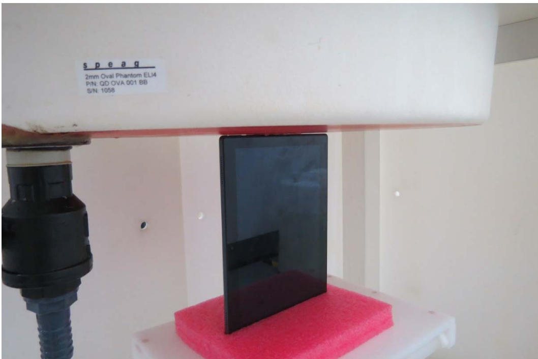
Picture 9: Right Side, the distance from handset to the bottom of the Phantom is 0mm
