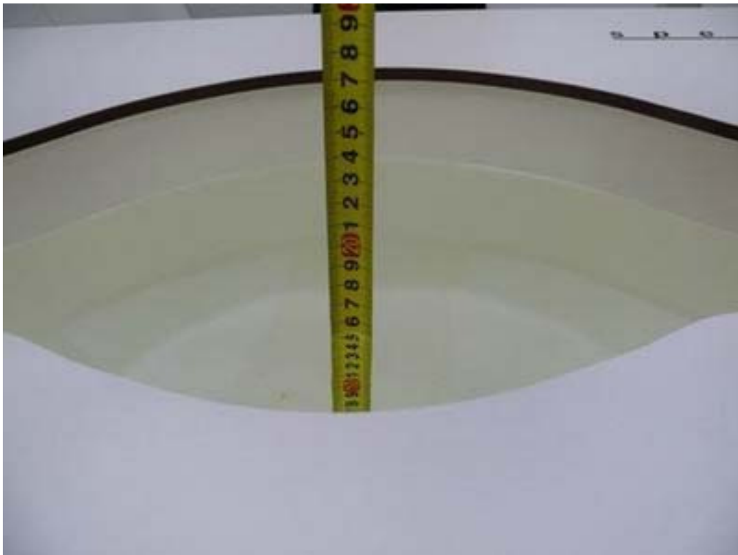
Picture 4: Liquid depth in the flat Phantom (5250 MHz, 15.3cm depth)
