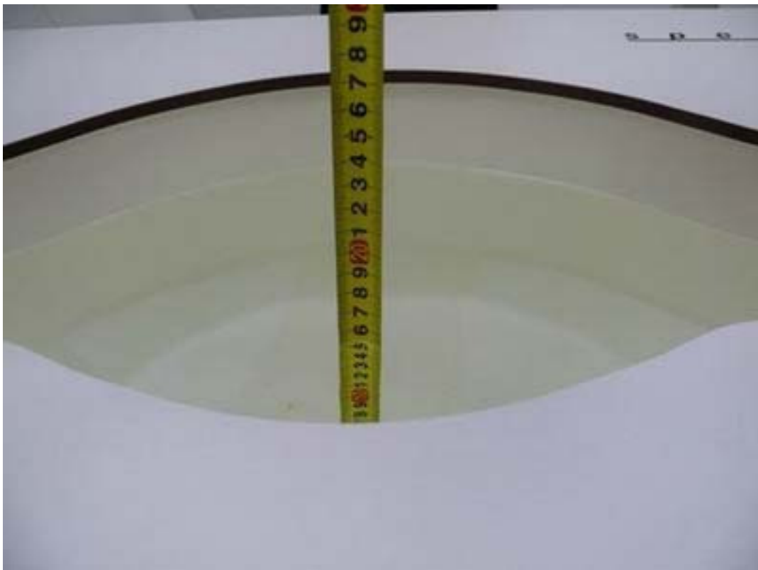
Picture 6: Liquid depth in the flat Phantom (5750 MHz, 15.0cm depth)
