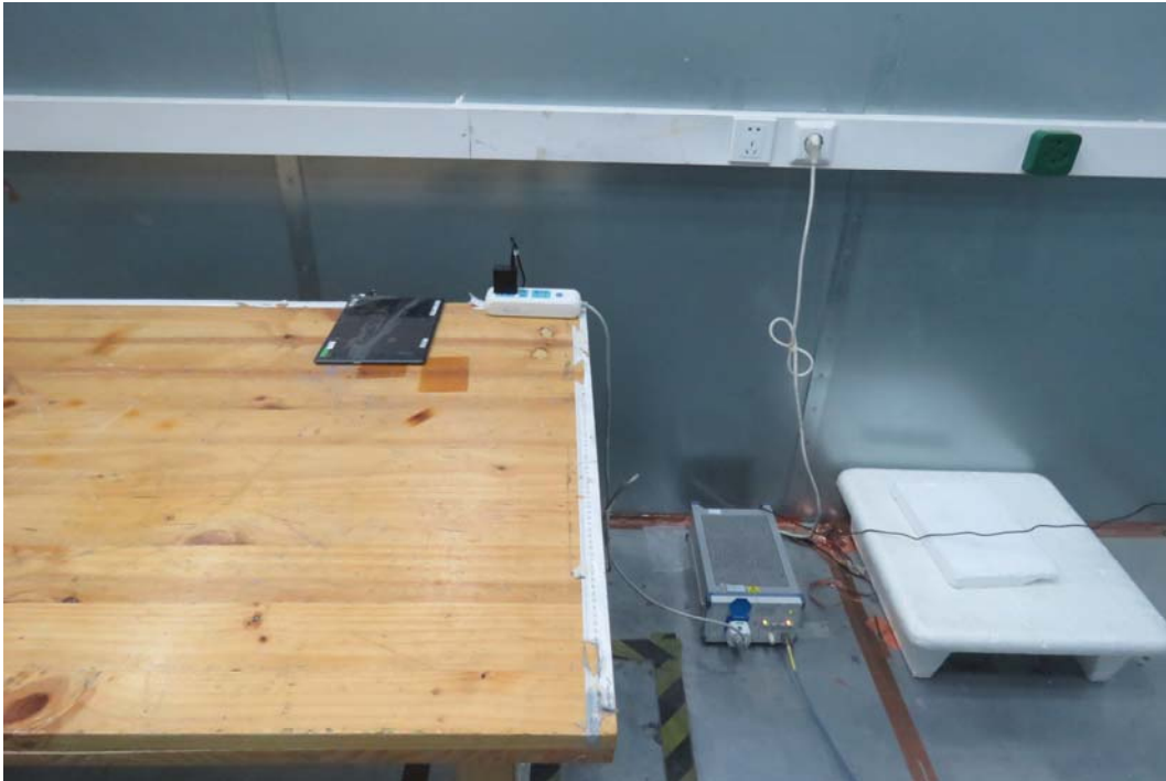
Picture 3 Conducted Emission Test Setup
