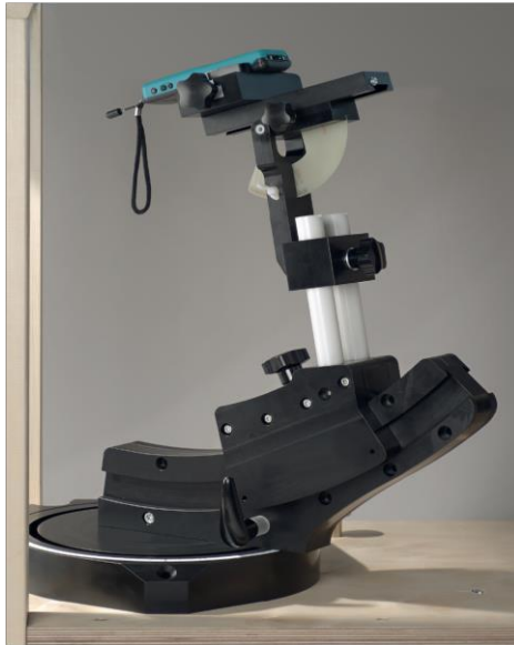
F-2. Device Holder for Transmitters
