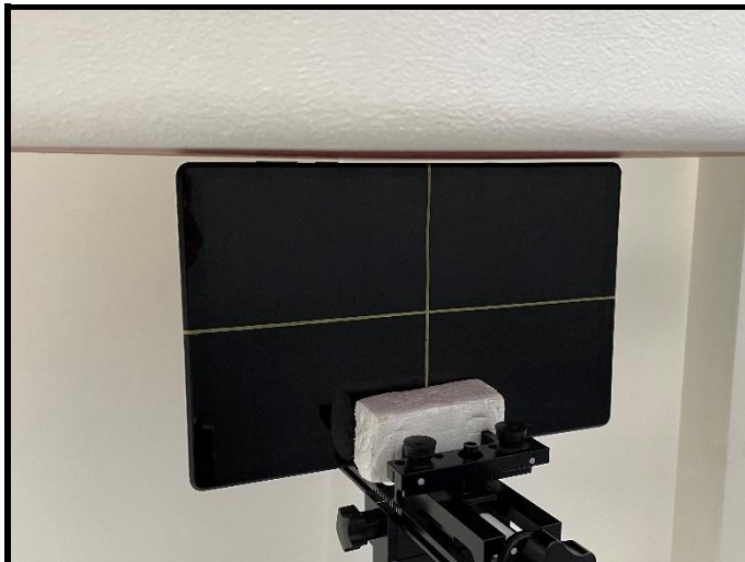
Right Side of EUT with 0.3 cm Gap
