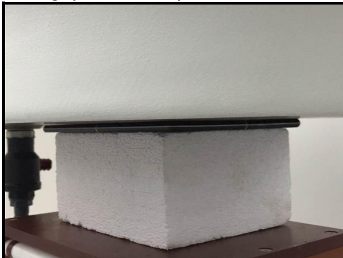
Rear Face of EUT with 0 cm Gap
