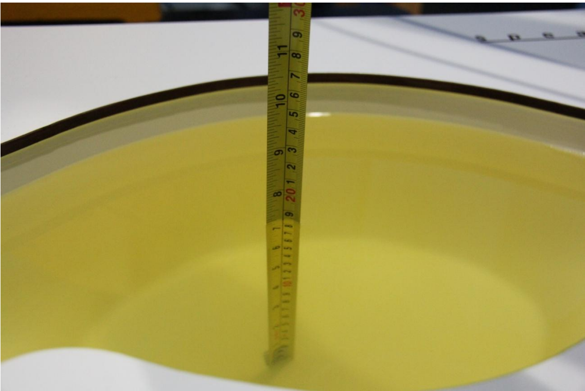
Picture 7-3 Liquid depth in the Flat Phantom (1900MHz)
