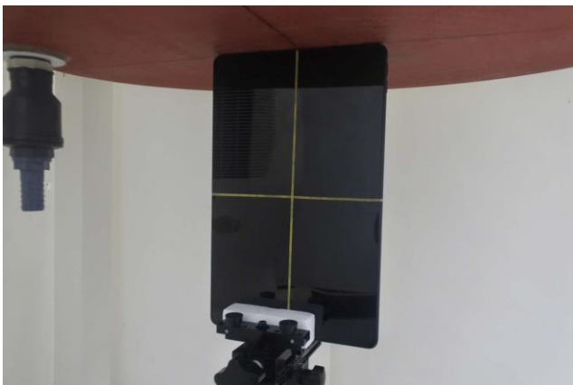
Edge 4 of EUT with Phantom 0 mm Gap
