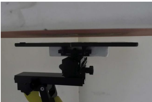
Bottom Face of EUT with Phantom 19 mm Gap (Sensor off) for Antenna 1
