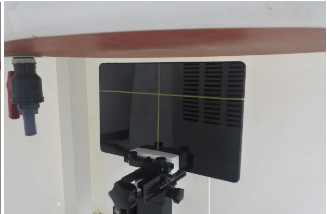
Edge 1 of EUT with Phantom 18 mm Gap (Sensor off) for Antenna 2
