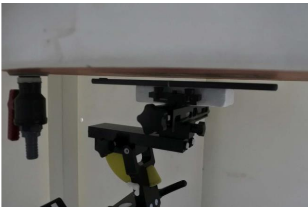
Bottom Face of EUT with Phantom 6 mm Gap (Sensor off) for Antenna 3
