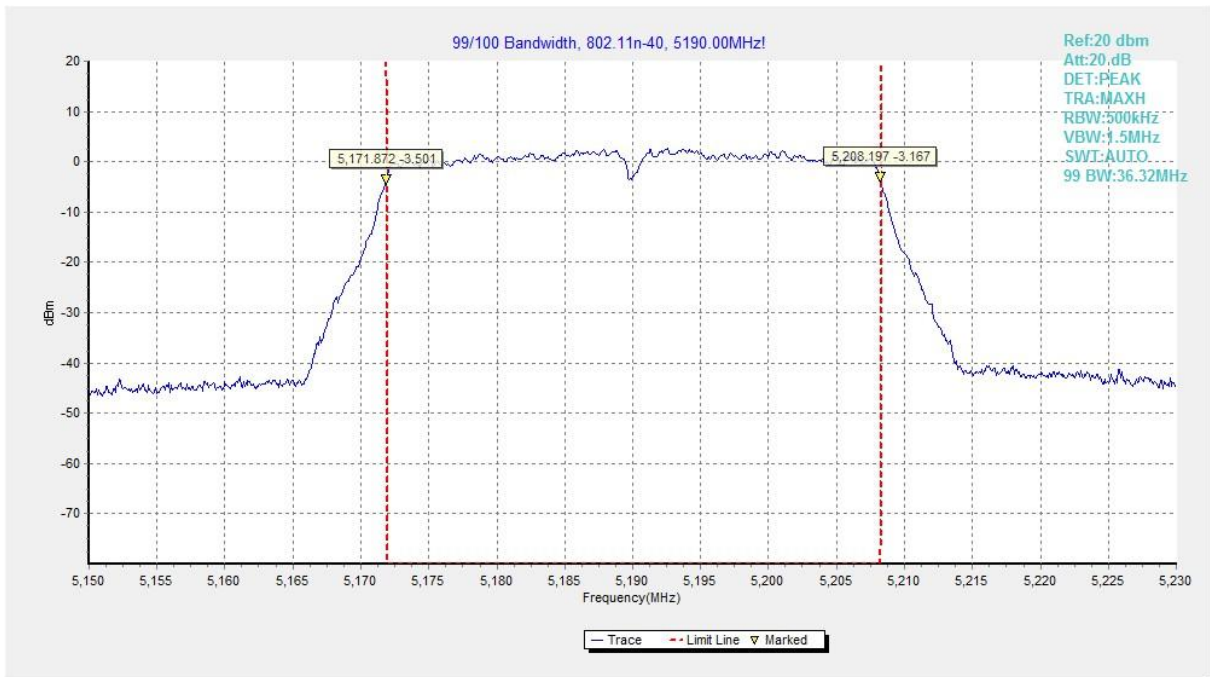
Fig.81 99% Occupied bandwidth (802.11n-HT40, 5190MHz)
