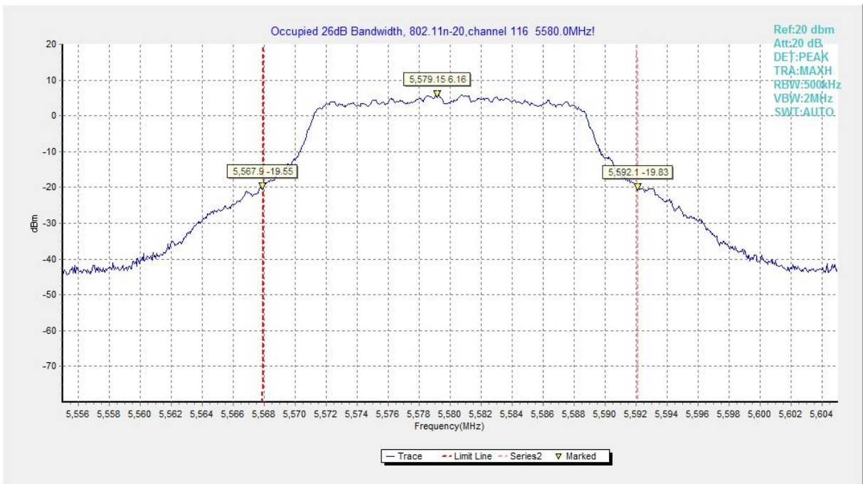
Fig.18 Occupied 26dB Bandwidth (802. 11n-HT20, 5580MHz)
