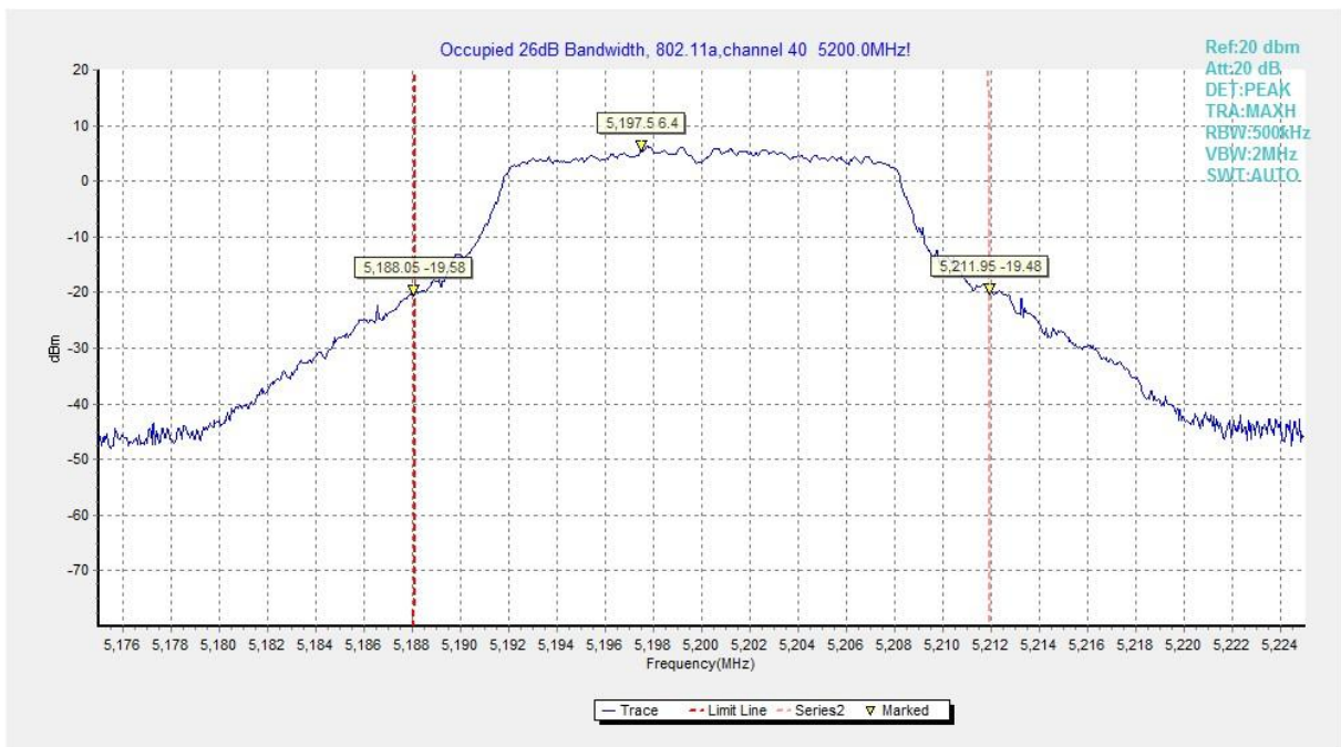
Fig.2 Occupied 26dB Bandwidth (802.11a, 5200MHz)
