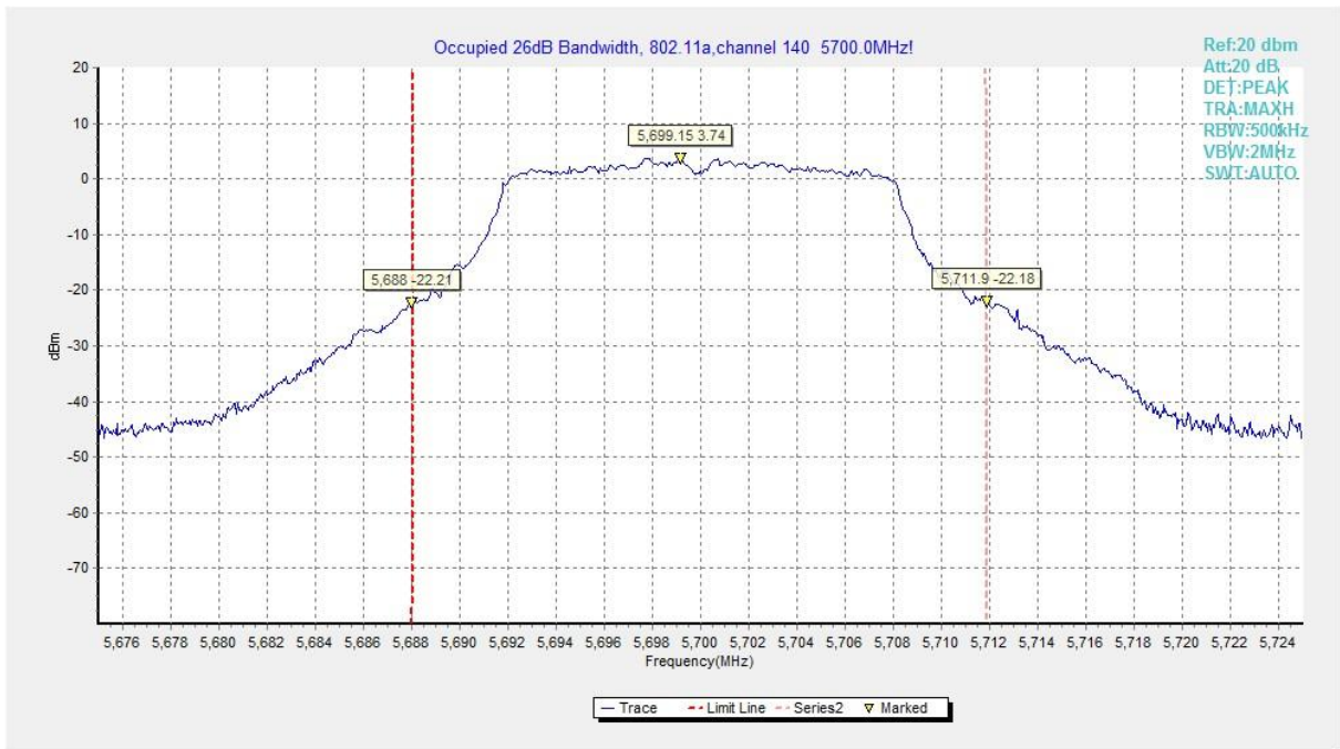
Fig.9 Occupied 26dB Bandwidth (802.11a, 5700MHz)
