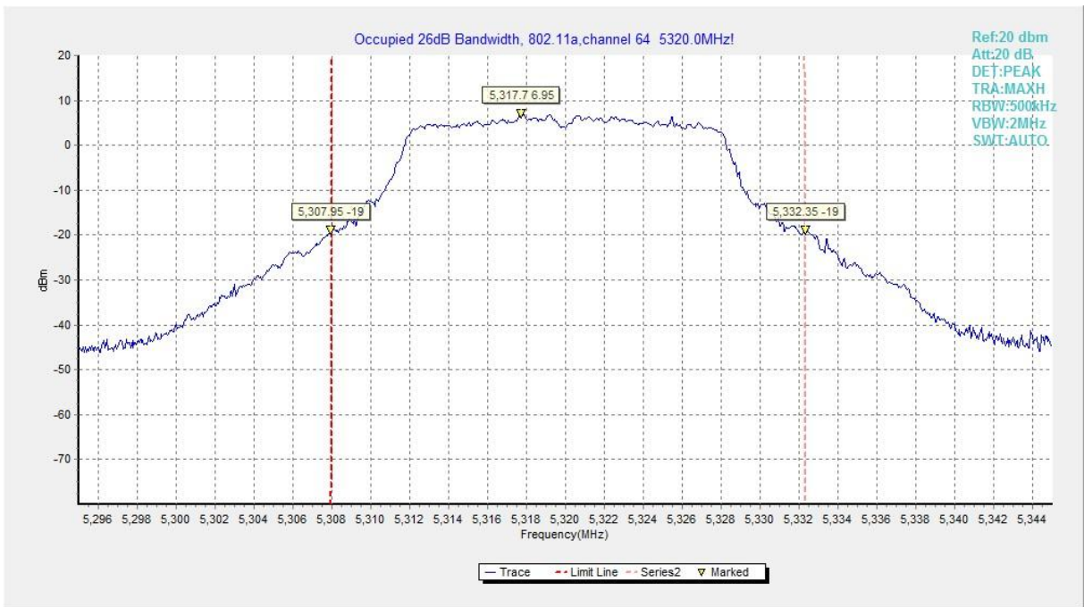
Fig.6 Occupied 26dB Bandwidth (802.11a, 5320MHz)
