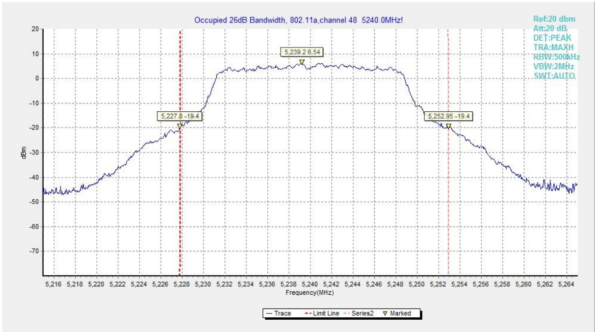
Fig.3 Occupied 26dB Bandwidth (802.11a, 5240MHz)
