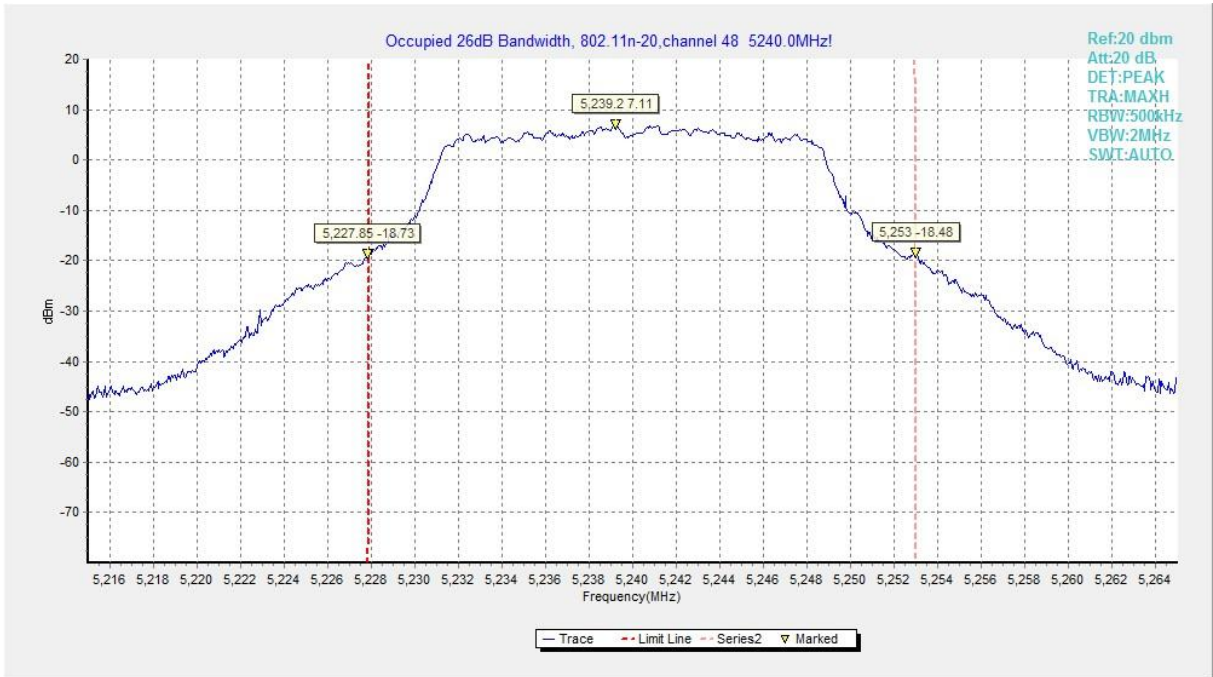
Fig.13 Occupied 26dB Bandwidth (802.11n-HT20, 5240MHz)
