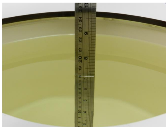
Fig 11.1 Photo of Liquid Height for Body SAR
