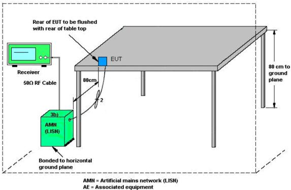
EUT = Equipment under test
